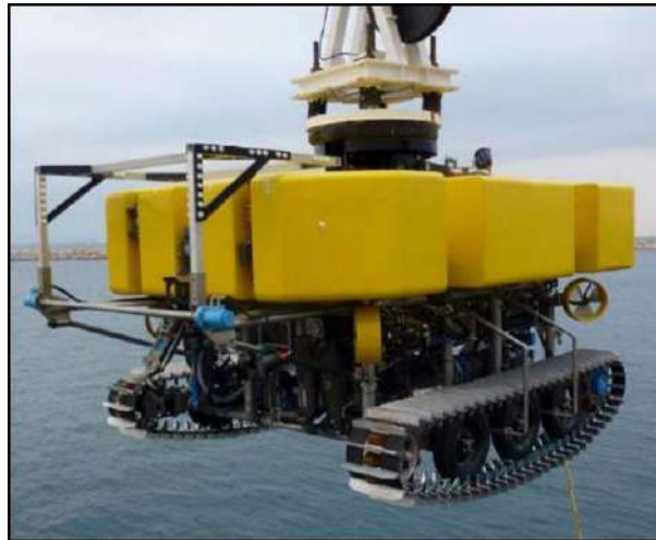
Figure 12 : Engin de water-jetting (RTE, 2021)
