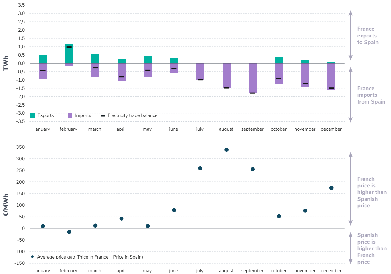
Figure 53: Electricity trade balance (top) between France and Spain and Average monthly gap between spot prices in France and Spain (bottom) in 2022, by month
