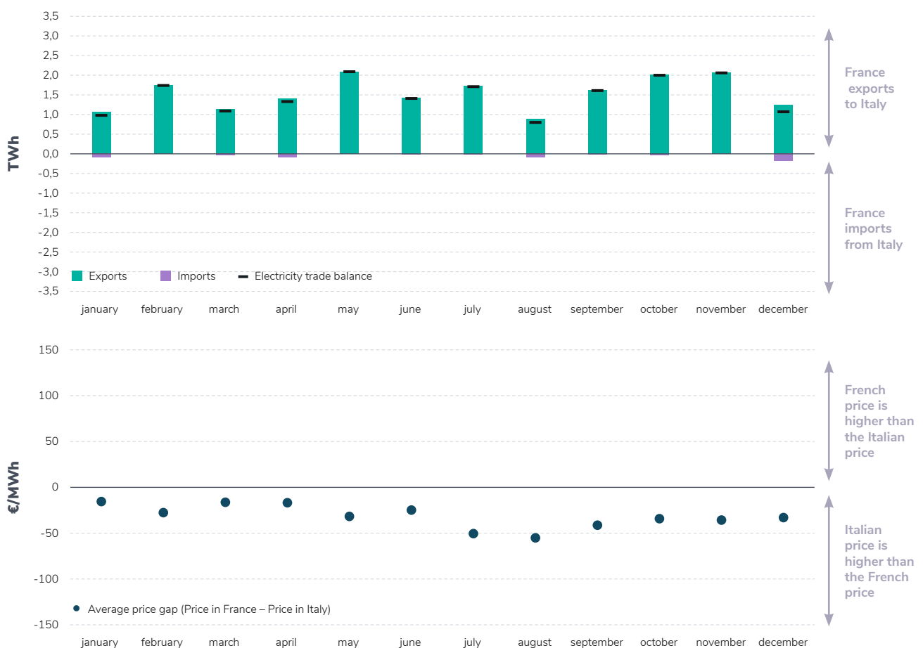
Figure 56: Electricity trade balance (top) between France and Italy in 2022, by month, and Average monthly gap between spot prices in France and Italy (bottom) in 2022, by month
